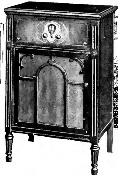
AN ALL-AMERICAN HIBOY The receiver employs six tubes, and may be obtained either to use the new a. c. tubes or for ordinary tubes, batteries or power units being required in the latter case
